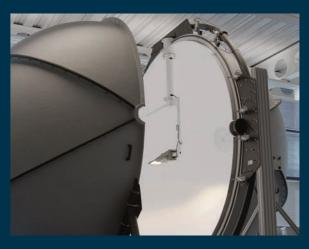
Our LED solutions have been fully photometrically tested within our luminaires, using our in-house goniophotometer and stateof-the-art integrating sphere.
