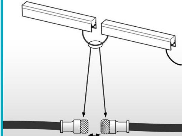
For ease of installation an IP68 twist connector is provided at each end for easy connection.
