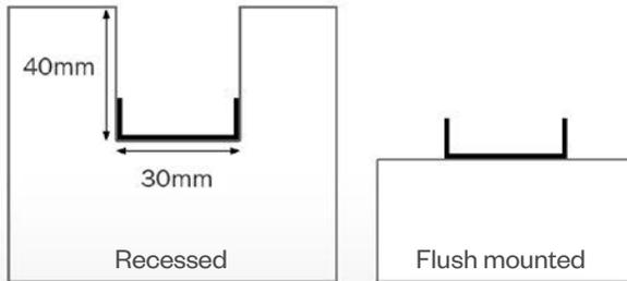
Vaio can be recessed or flush mounted as shown above.
