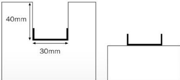
Vaio can be fitted 'inground' or 'flush' as shown above
