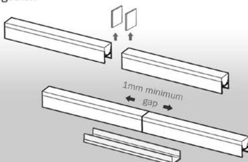
5 Fix Vaio into place by pushing it down onto its mountings. Make sure that cables are not crushed during this process. Use a suitable sealant or grout to finish off the surface.
