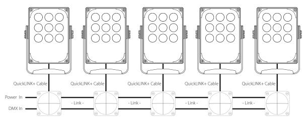
LuxCONNECT IP66 Hardwired connection boxes with combined Power & DMX wiring & QuickLINK+ luminaire connections
