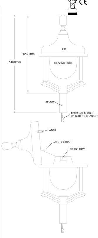
DIAMETER = Ø652mm WEIGHT = 24.3kg
