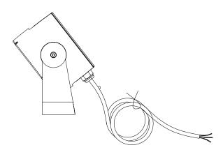
1.5mm<sup>2</sup> 3-core cable (on/off version) 1.5mm<sup>2</sup> 5-core cable (DALI version) All supplied pre-cabled
